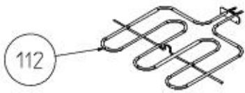
TOP AND GRILL HEATING ELEMENT (OPTIONAL ONLY FOR ELECTRIC GRILL NEW G.FS GAS)
