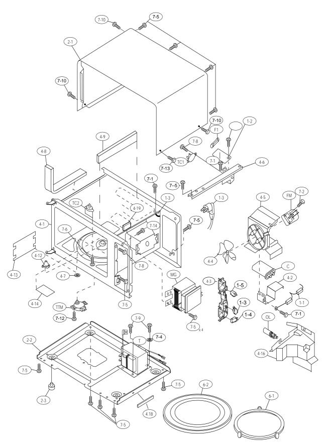
NOTE: In the event of removing the turntable motor cover this part should be refitted using screw connection: LX-EZA045WRE0 (7-11)
