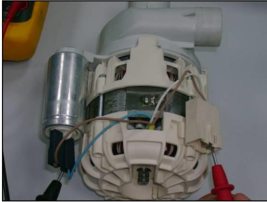
Measurement of the primary winding
